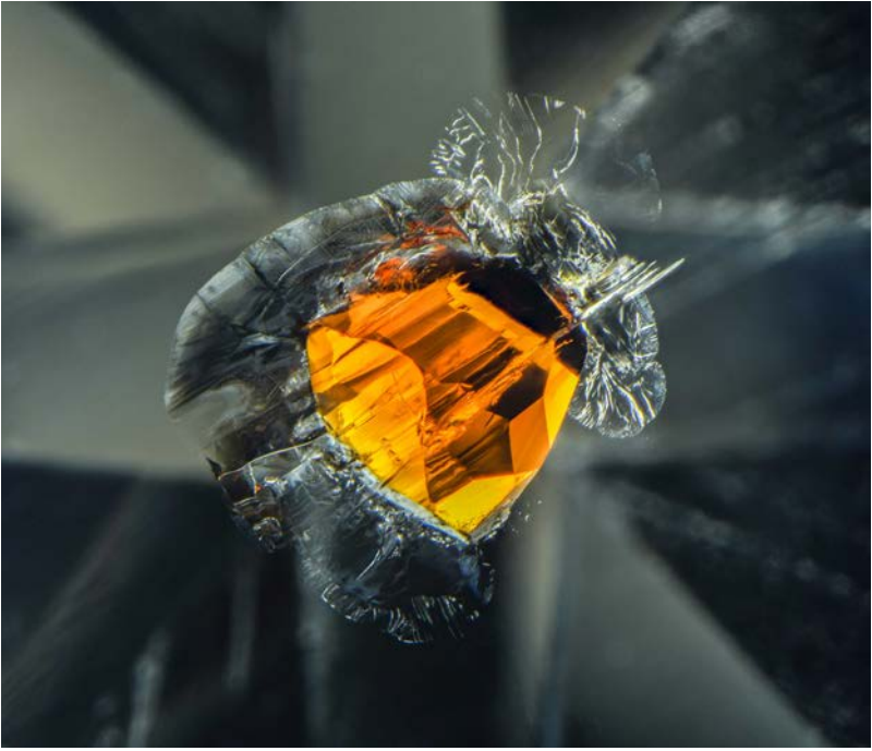
This garnet inclusion shows up as a bright orange crystal in its quartz host when viewed using darkfield illumination.
