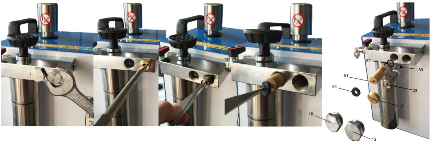
FIG 4 – CHECK VALVE AND BACK FLAME FILTER REPLACEMENT
